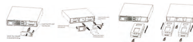
Easy for maintenance, hot-swappable battery
